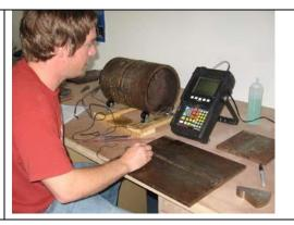
UT Equipment and welded test samples available for the UT II class. (a) USM36, USMGo, USN 60, Epoch 600 (b) practicals on welded test samples with embedded flaws
