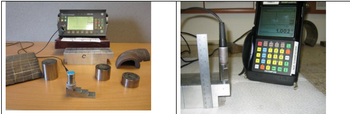
UT I Practical Training (a) Various test samples (b) measuring thickness on a Aluminum Block
