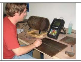
UT Equipment and welded test samples available for the UT II class. (a) Epoch 4, USN 60, USN 58, USN Go, Epoch 600 (b) practicals on welded test samples with embedded flaws
