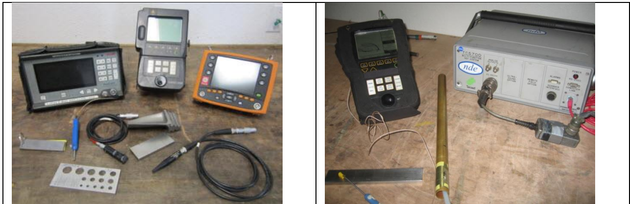
Eddy Current Equipment (a) Surface inspection Hocking, Nortec 1000, GE Phasec 3D (b) Nortec and TC 5700 for Tubing
