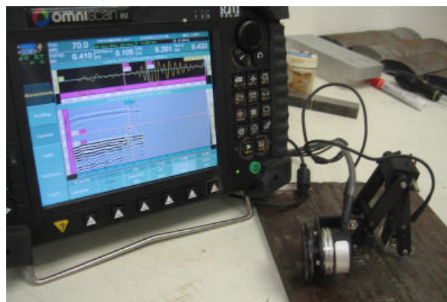
Basic TOFD Setup on a Omniscan
