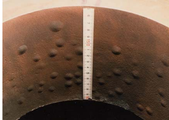
Figure 2 Blistering observed on C-0.5Mo nozzle flange used in Platformer unit
